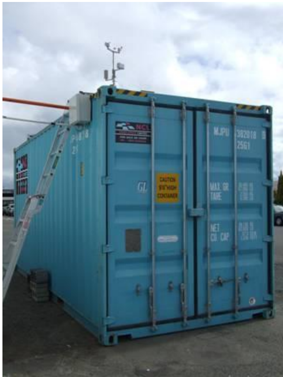
Figure 3.1: Shipping container used for ambient heat loss tests.
