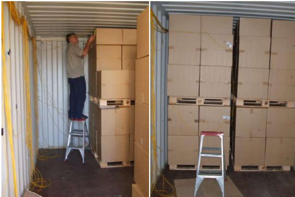
Fig. 3.6: Stacking pallets and placing thermocouples, and the arrangement of the load on pallets.
